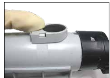
14. Press down until the tabs lock it into place.
