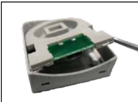
11. Carefully lift the chip from its housing.
