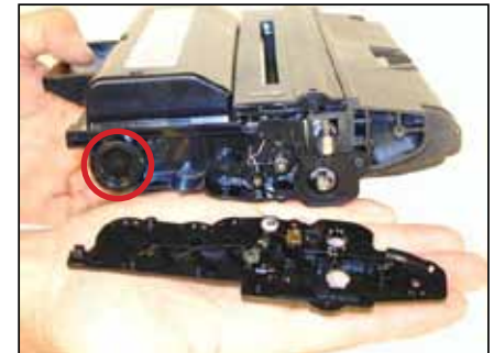
D. Remove plug (circled in red) and remove any remaining toner before refilling.
