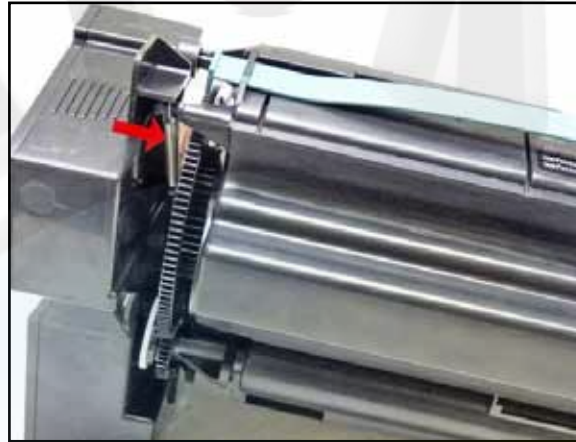
Remove the spring on the inner part of the cartridge.
