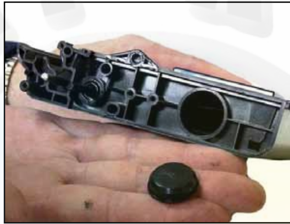
Remove the toner hopper plug, dump out and discard of any old toner before refilling with new toner.
