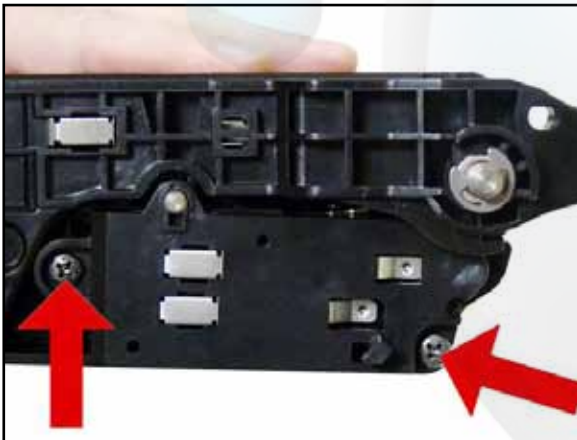
Remove screws holding down the contact plate.
