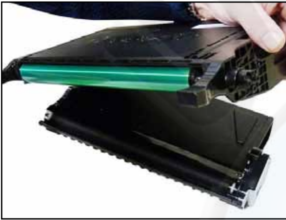
Pull apart the two halves of the cartridge.
