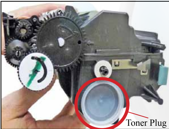
Locate the Toner Plug, and carefully remove it from the cartridge. Remember to dispose of any toner left inside the compartment before refilling.
