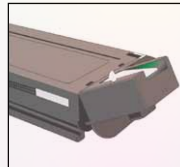
Remove handle assembly carefully
